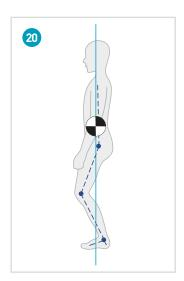
The patient is standing on the h-cast. Adjust it so that all influencing factors, such as extension limitations, are taken into account. Drop the plumb bob from the centre of gravity to determine whether the plumb line runs behind the knee's pivot point.
