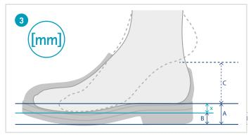
Determine pitch x of the shoe (difference between heel height A and sole thickness B in the ball area). Measure A and B and apply the formula x = A - B. Transfer the determined pitch to the h-Cast.
