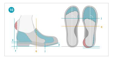
When producing a height compensation, it is essential to create a leverage ratio that is similar to the contralateral side. To do so, the following steps are necessary:
