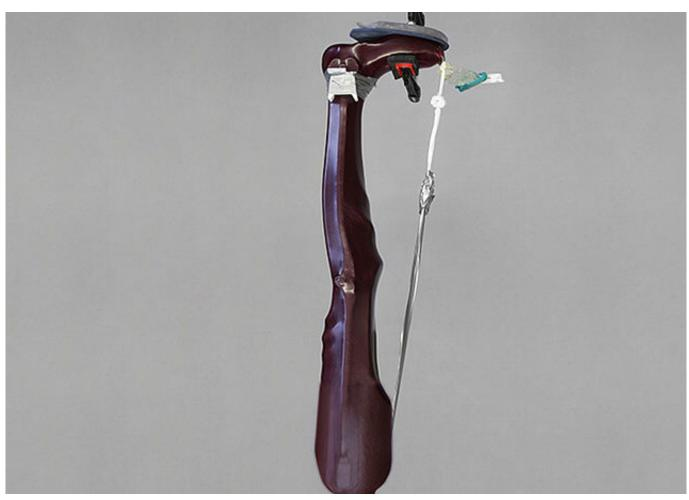
Leave the model overnight (at least 10 hours) under vacuum at room temperature. Important! Follow the processing instructions for the epoxy resin here as well.
