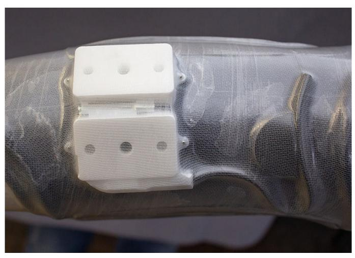
Remove the system string. If the model is still wet, insulate it with compression film. Then, pull a PA reinforcement stocking and a PVA film tube over the model. The lamination dummies for the controller and the connection cable are now located under the PVA film tube and are thus part of the model.
