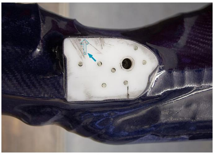
Cut the system joints free. An arrow is milled on the assembly/lamination dummy to indicate where to lever out.
