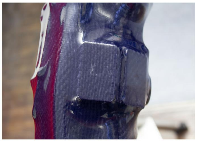
For this step, the laminate in the area of the lamination dummy for the controller remains closed. Saw the orthosis shells and remove them from the model. The lamination dummy for the controller and the lamination dummy for the cable length compensation remain on the model for the time being.
