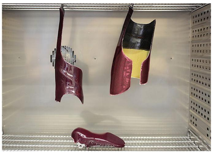
Clean the orthosis shells and remove the PVA film tube. Temper the orthosis shells. Important! Follow the processing instructions for the epoxy resin here as well.
