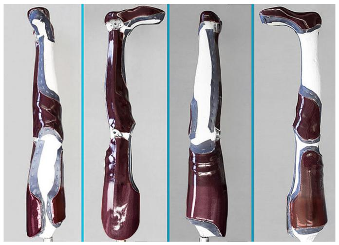
Remove all laminate parts which are no longer necessary. Then, you can remove the orthosis parts from the model.
