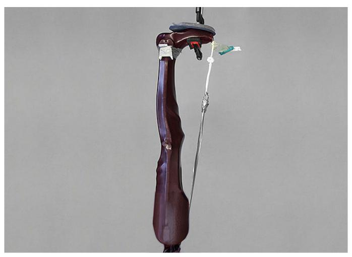
Let the model harden over night (at least 10 hours), under vacuum and at room temperature.
