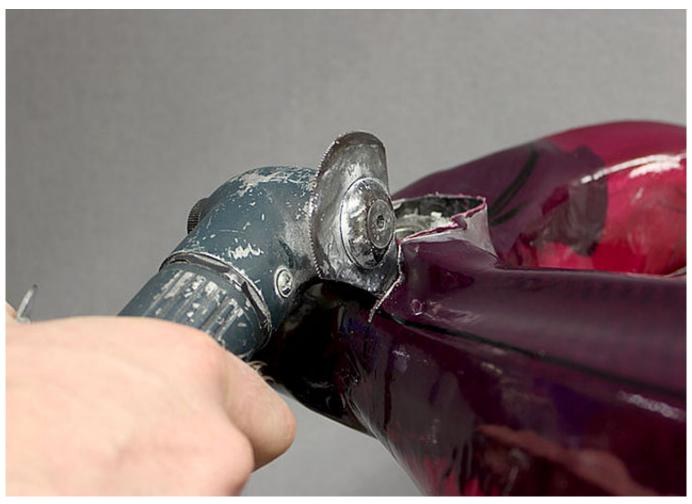
Use an oscillating saw to saw along the cutting edges in order to remove the orthosis parts from the model. You can see the recommended saw blade in the picture. Thus, you can saw very close to the system joint without damaging it.
