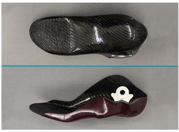
Grind the edges of the orthosis parts (e.g. with a belt grinder).
