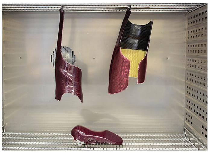
Temper all orthosis parts before grindig them. Place the orthosis parts into a cold convection oven and heat it up slowly. When tempered, the orthosis parts are stable and can be worked in the best possible way.
