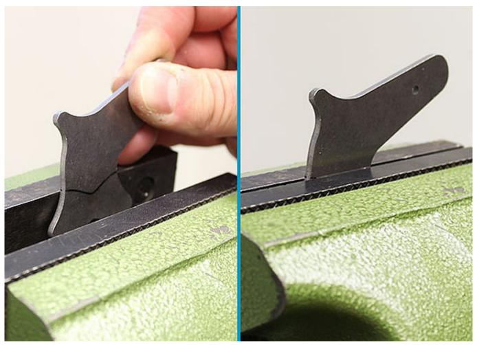
Clamp the system stirrup into a vice with plain jaws to bend it. Pay attention to the marking to avoid a subsequent deformation of the joint areas and to be able to bend very close to the joint. *Note: When you have acquired a bent system stirrup, you can skip the steps 2 to 4.*
