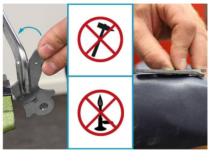
Adapt the system stirrup to the shape of the model. Bend the lower part of the system stirrup with a bending iron. Only bend in one direction.
