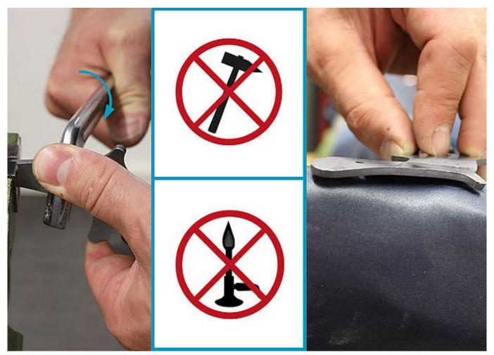
Adapt the system stirrup to the shape of the model. Bend the system stirrup foot with a bending iron. Only bend in one direction.
