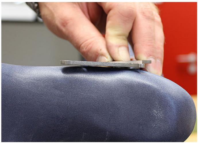
Remove the system stirrup from the vice and check the distance from the system stirrup to the model. *Note: When you have acquired a bent system stirrup, you can skip the steps 2 to 4.*
