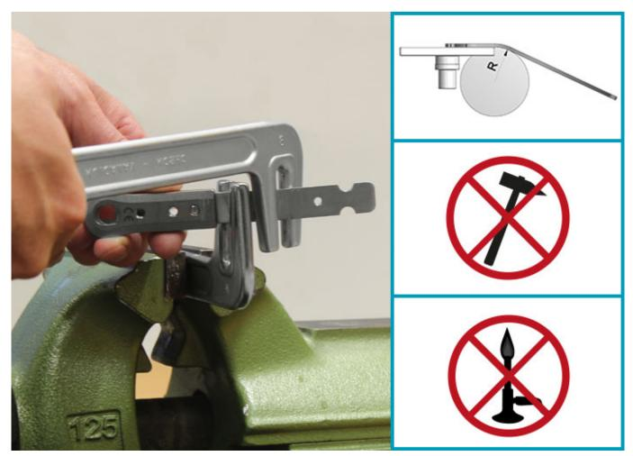
While bending, please consider the applicable bending radii and use a bending iron with round edges. *Note: You will find information on bending radii and the tools to be used in the* instructions for use.
