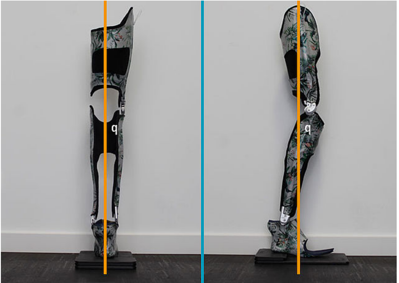
Finally assembled orthosis with height compensation View: posterior, lateral
