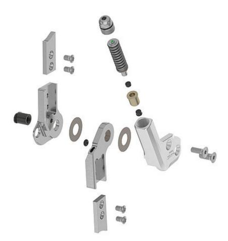
Disassemble and clean the system joint. In order to clean the threads in the cover plate, use Super Clean LOCTITE<sup>®</sup> 7063 to remove any insulating wax residues. *Note: mind the* safety data sheet *when using Super Clean LOCTITE<sup>®</sup> 7063.*
