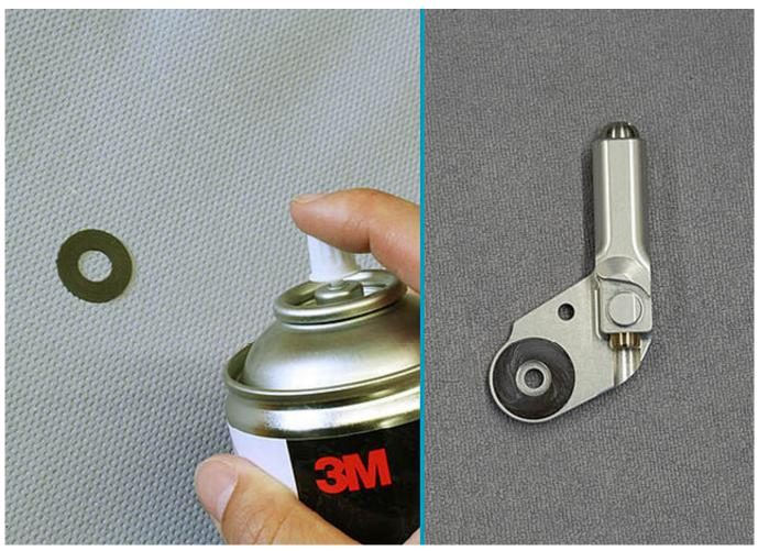
Apply spray adhesive to one side of the first sliding washer and adhere it to the cover plate. Grease the other side of the sliding washer slightly with orthosis joint grease.
