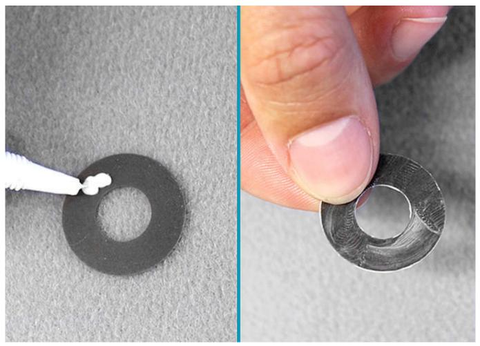
Grease the second sliding washer slightly with orthosis joint grease.
