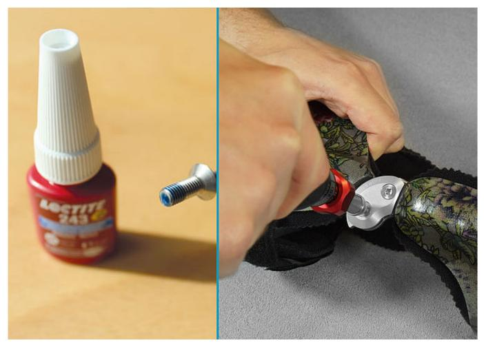
Secure both screws with LOCTITE<sup>®</sup> 243 medium strength and the torque corresponding to the system width. Let the adhesive harden (final strength after approx. 24 hours). *Note: mind the* safety data sheet *when using LOCTITE*<sup>®</sup> *243 medium strength.*
