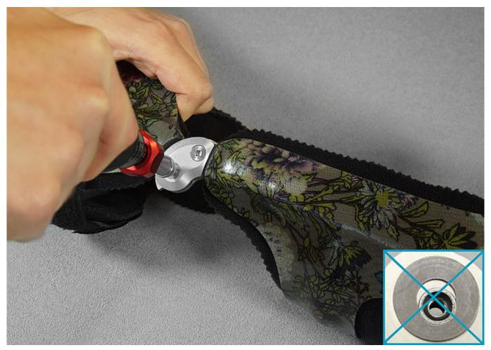
Make sure not to damage the sliding washer during assembly. Jammed sliding washer particles can cause lateral play in the system joint.
