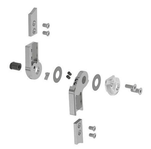
Disassemble and clean the system joint. In order to clean the threads in the cover plate, use Super Clean LOCTITE<sup>®</sup> 7063 to remove any insulating wax residues.
