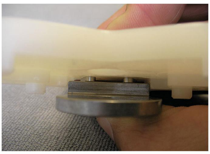
Place the assembly/lamination dummy onto the joint's upper part in such a way that the feather keys with pin are inserted into the grooves.
