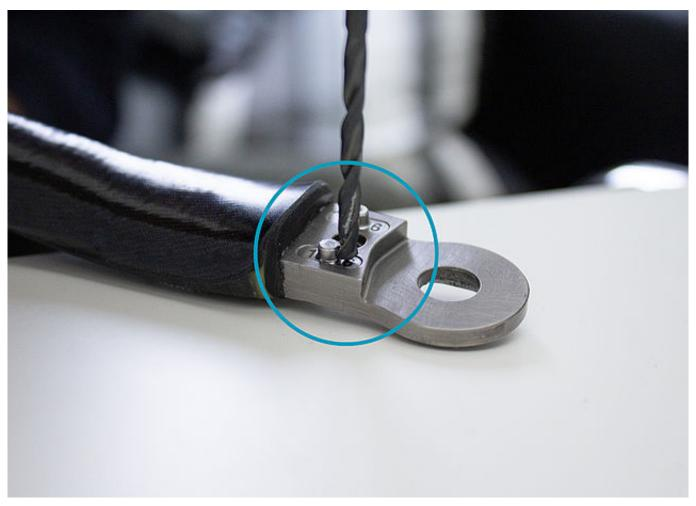
Remove the defect feather keys with pin by boring them out with a small drill.
