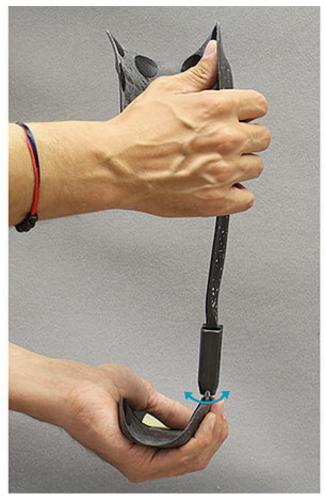
Hold the lower leg shell and try to move the foot shell in pronation-supination direction. If there is lateral play, this can indicate loosened screws and/or worn out sliding washers.
