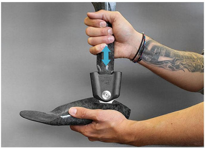
Check if there is play around the axis. If there is play, the bearing nut and the sliding bushing should be replaced if necessary.
